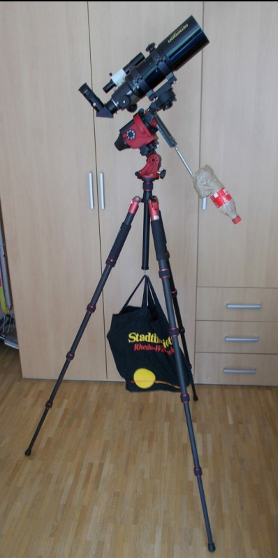
The optic is a small 80mm f/5 Fraunhofer made in China . The weight is much smaller as the weight of my 72mm Apochromat and for occultations no high magnification is needed. An advantage is the finder-shoe.
